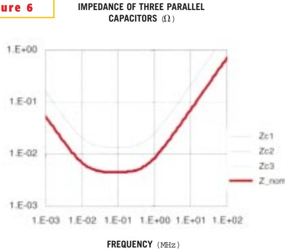
**Tantalum capacitors exhibit three distinct impedance regions. At low frequencies, they appear capacitive. At high frequencies, they appear inductive. In a middle range, they appear resistive. This plot shows the impedance versus frequency of three T510 devices—individually (upper curve) and in parallel (lower curve).**
