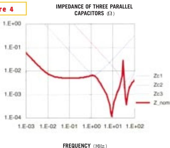
The impedance of this parallel combination of three types of capacitors is well-behaved at frequencies below 1 MHz. At higher frequencies, you see series-resonant valleys and parallel-resonant peaks. These devices have low ESR and relatively high ESL. The three types are 330  $\mu$ F tantalum (eight in parallel), 0.22  $\mu$ F ceramic chip (100 in parallel), and 0.01  $\mu$ F ceramic chip (100 in parallel). The two types of chip capacitors have an ESL of 1.5 nH.
