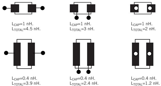
The way you route the power and ground connections to a surface-mounted chip capacitor can cause the mounted device's wiring inductance to vary from 0.8 to 3.5 nH, a range of 4.375 to 1.
