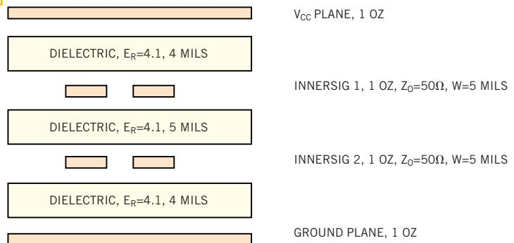
In this four-layer pc board, the power plane is on top, the ground plane is on the bottom, and the signals are on the two inner layers. You see an end view of two side-by-side striplines, both of which lie between the plates of the capacitor that consists of the power and ground planes and the dielectric material between them.
