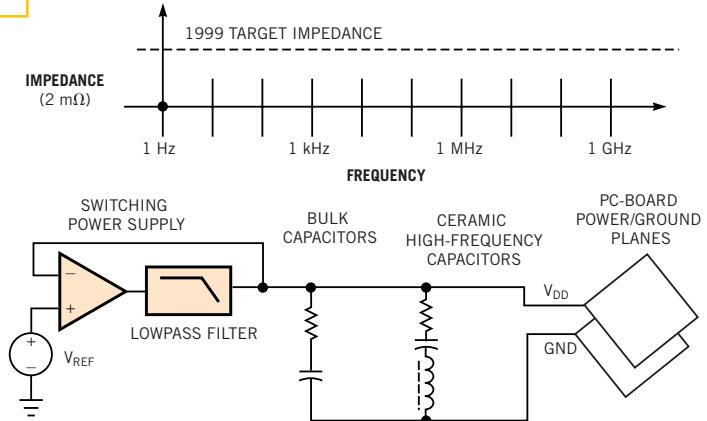
For the purposes of signal-integrity analysis, a power-distribution system comprises the power supply, "bulk" electrolytic capacitors, ceramic-chip capacitors, and the power and ground planes within the pc board.
