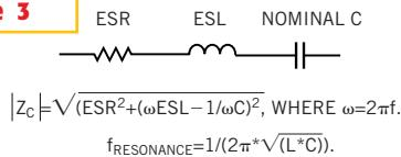
This capacitor-equivalent circuit consists of three elements in series—the device's nominal capacitance, its ESL, and its ESR. Sometimes, you see the circuit drawn with another element—a conductance shunting the capacitor. In some cases, that shunt conductance is frequency-dependent.
