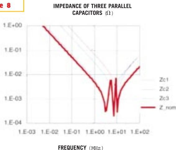
**Selecting low-ESL capacitors does no good unless you mount them properly. The inductance of the connections to the power and ground planes ruins the behavior of these devices.**
