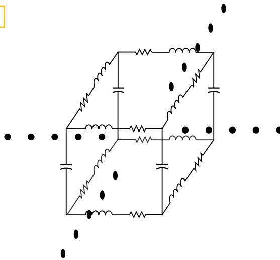
**You can regard power planes as distributed networks containing shunt capacitance and series resistance and inductance. Shunt conductance across the capacitance is also present, but its effects are usually negligible.**
