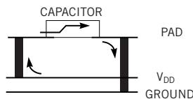
**As this cross-sectional view of a mounted chip capacitor shows, the path that the current follows from  $V_{CC}$  or  $V_{DD}$  to ground can be substantial, thanks simply to the placement of the power and ground planes near the board surface farther from the capacitor. The ESL of the mounted device depends strongly on the area of this loop.**
