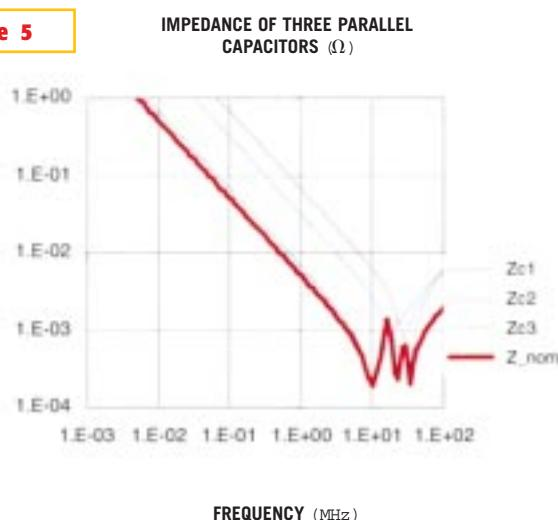
Selecting capacitors for lower ESL than those in **Figure 4** allows you to use fewer devices and to achieve a lower impedance over a broader range of frequencies. This setup uses chip capacitors whose ESL is 0.5 nH (50 units of each of three values: 0.47, 0.1, and 0.047  $\mu$ F).
